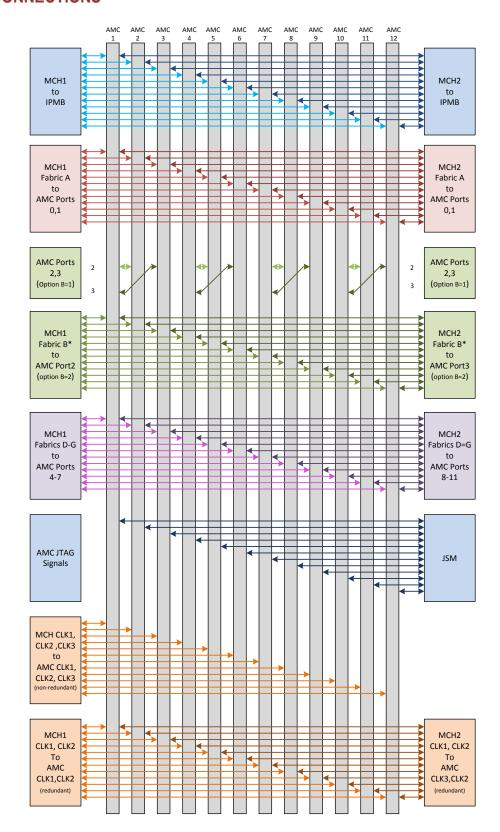
\*When CLK3 is non-redundant, Fabric B will be partially provided only on ports 1 to 6. CLK3 is routed on Fabric B on ports 7 to 12.
